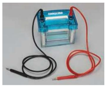
213713 Carolina Vertical Dual Gel Electrophoresis Chamber
