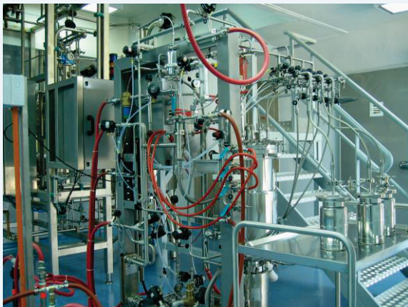
500Litre Bioreactor used in production of R.anatipestifer & P. multocida at the Veterinary Research Institute Malaysia.
